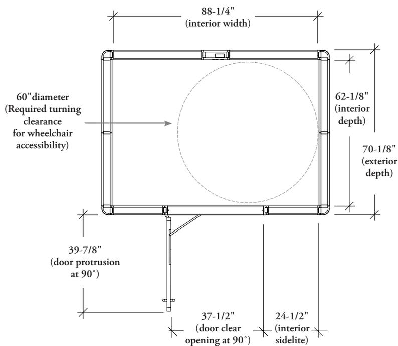
Tek Room's orientation is determined by the handedness of the pivot door as viewed from the front exterior. Tek Room's door pivots open to the exterior only.
