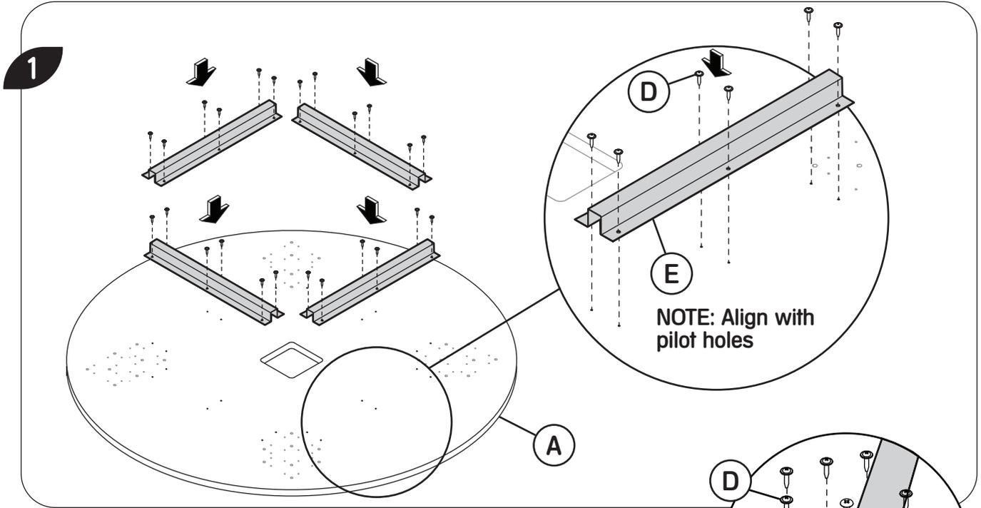
NOTE: Place the Table Top on a clean surface, underside facing up.
