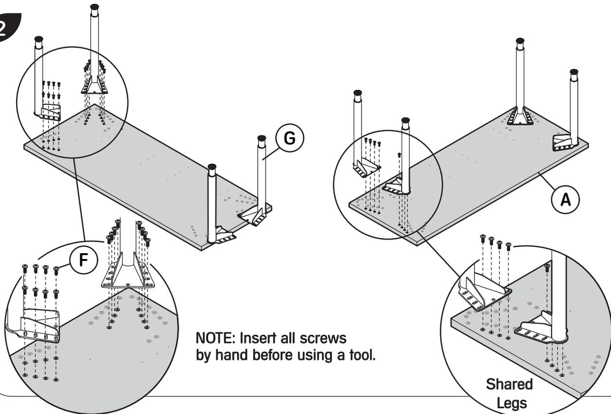
NOTE: Insert all screws by hand before using a tool.
