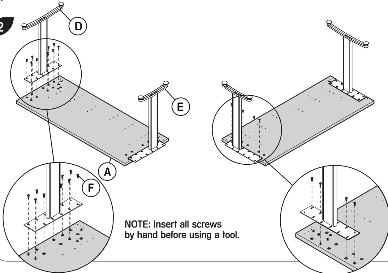
**NOTE:** Insert all screws by hand before using a tool.
