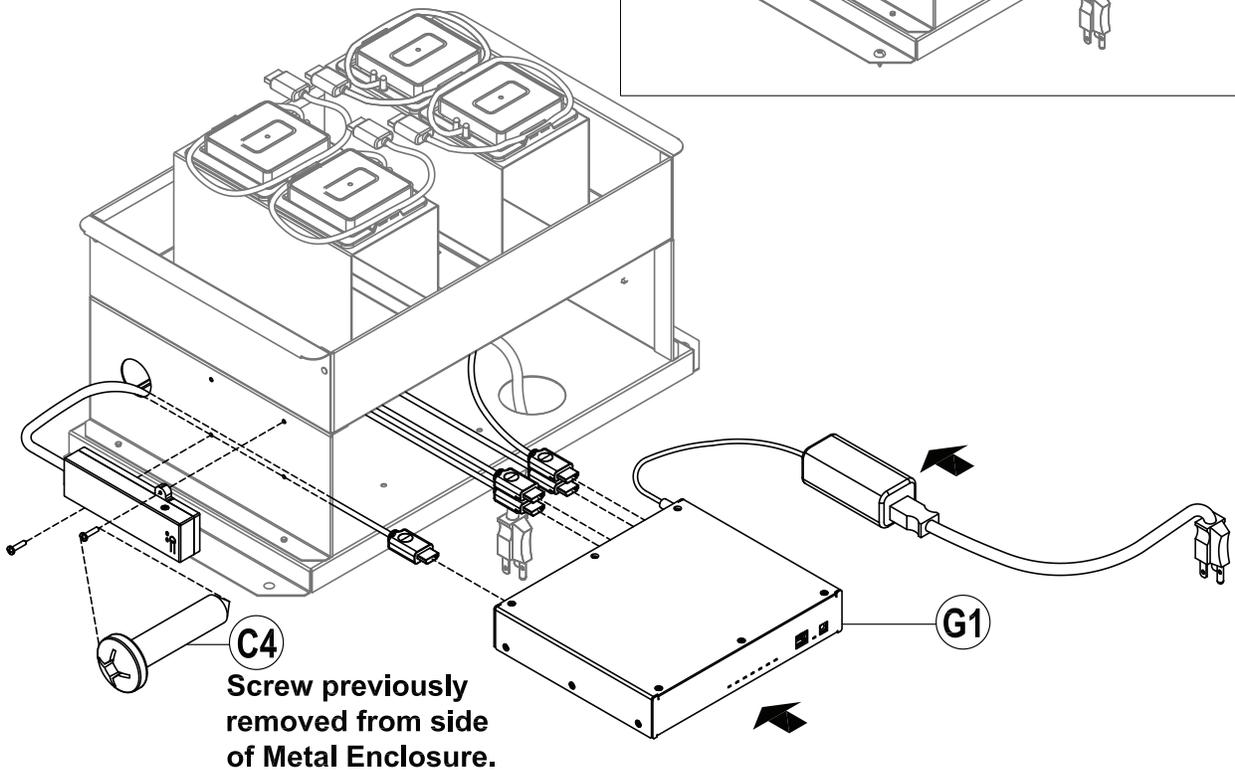
**Screw previously removed from side of Metal Enclosure.**
