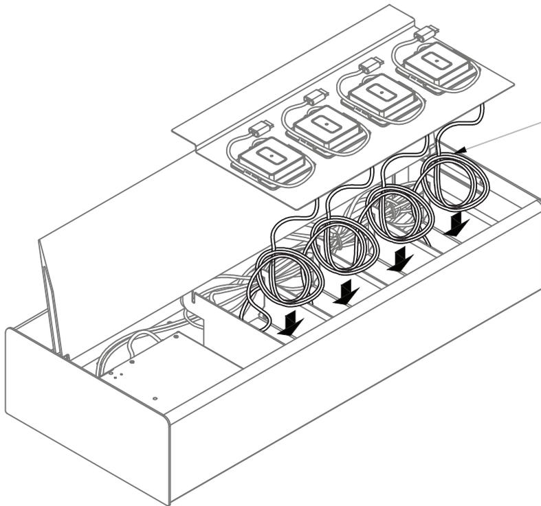
Coil cable inside each corresponding slots.
