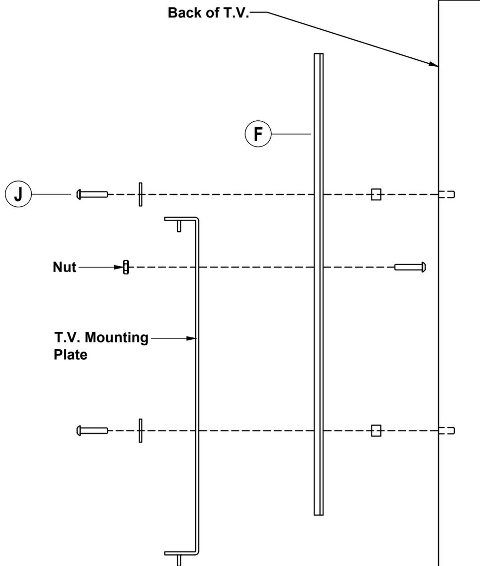
**NOTE: Follow illustration above if Mounting Plate does not cover mounting inserts at back of T.V. Skip to Step 21 if not applicable.**
